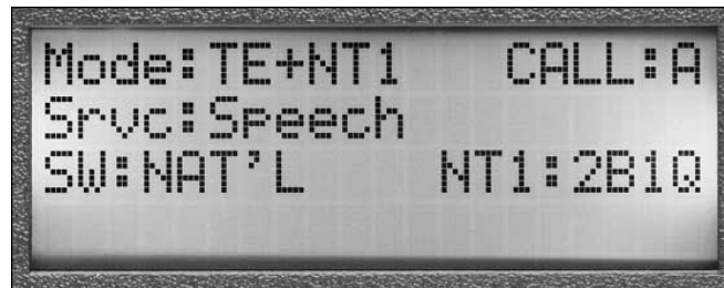
The CT-100's Home screen displays the current instrument operating mode – in this case, the CT-100 is functioning as both the TE and NT1.
