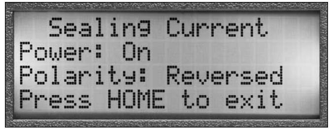
Figure 3. Checking for sealing current to verify an ISDN connection.
