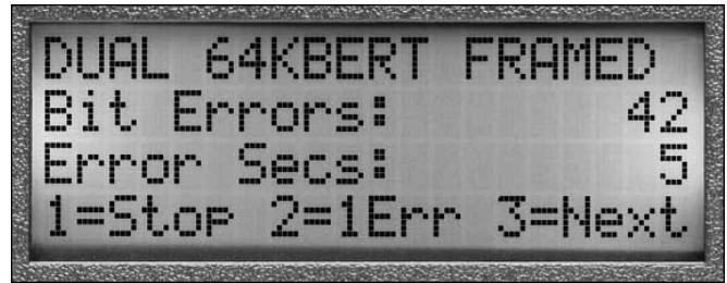
Figure 12. Monitoring bit errors using the CT-100's integrated BER testing.
