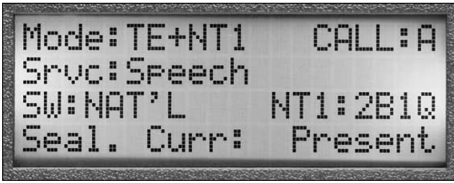
Figure 2. The presence of sealing current indicated in the home display.
