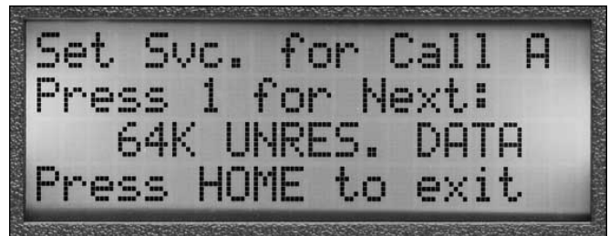
Figure 10. Verifying a circuit-switched data call involves selecting a new bearer service.
