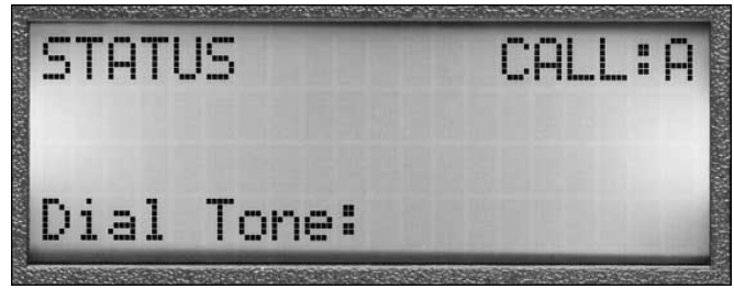
Figure 6. The CT-100 has received an acknowledgement, turning on dial tone.
