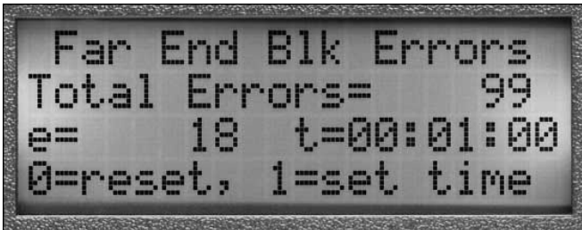
Figure 13. After running for one minute, 99 block errors were detected (18 errored seconds).
