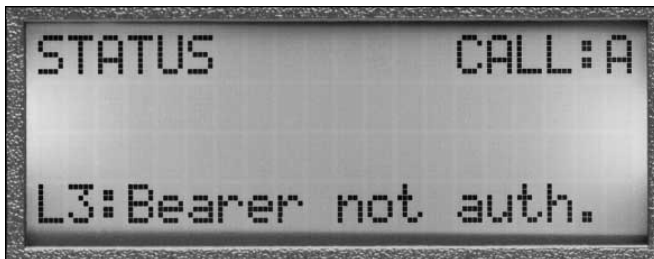
Figure 9. The requested bearer service is not authorized for the line (in this case, a circuit-switched data call was requested on a line provisioned for voice calls only).
