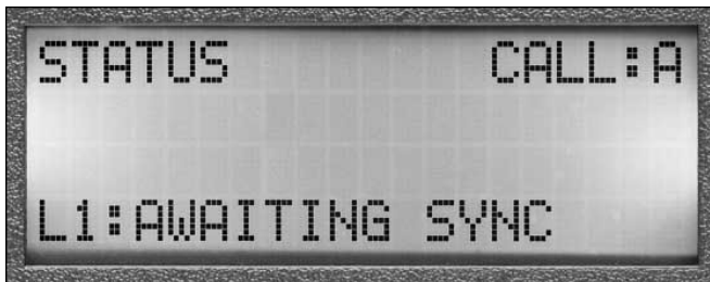
Figure 7. In addition to colored LED status lights, call progress is also indicated when off-hook.
