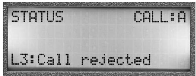
Figure 8. The call setup request was rejected, in this case due to an invalid SPID entry (National switch).
